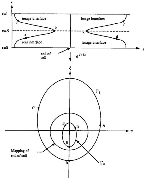
FIG. 2. The interface and its image system in the  $(x,y)$  and  $(\eta,\xi)$  planes. Corresponding points are indicated by upper and lowercase letters.
