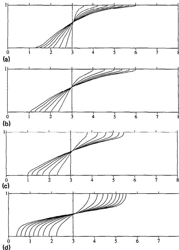
FIG. 4. Numerically generated interfacial profiles for different values of the nondimensional surface tension  $\tau$ . The initial interface is a vertical line at  $y = 3$  and the  $x$  coordinate has been magnified by a factor of 2. (a)  $\tau = 10^{-5}$ ,  $\Delta t = 0.11$ ; (b)  $\tau = 10^{-4}$ ,  $\Delta t = 0.18$ ; (c)  $\tau = 10^{-3}$ ,  $\Delta t = 0.3$ ; and (d)  $\tau = 10^{-2}$ ,  $\Delta t = 0.5$ .
