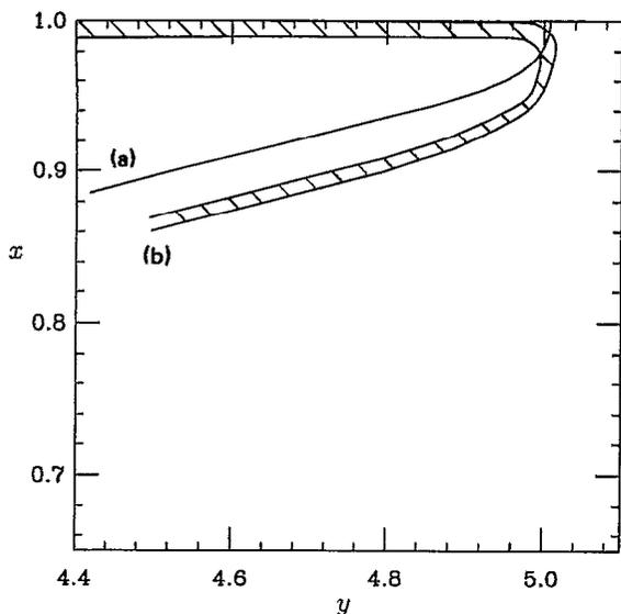
FIG. 6. Enlargement of Fig. 5(b) near the top edge of the cell. (a) numerical; (b) experimental;  $\mu = 13$  P. Illustration of the local deviation from the Hele-Shaw model.
