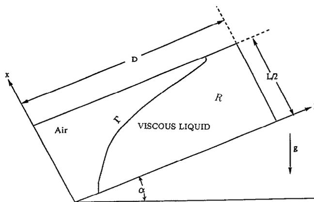
FIG. 1. Hele–Shaw cell oriented with the plates parallel to gravity and the long axis of the cell at angle  $\alpha$  to the horizontal. The two plates are separated by a distance  $b$  (into page).
