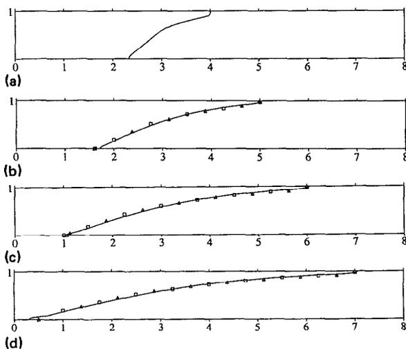
FIG. 5. Comparison of numerically predicted interfacial profiles, at various times, with experimental results, for  $\alpha = 0$ . The cell is filled with castor oil.—, numerical ( $\tau = 1.0 \times 10^{-4}$ );  $\square$ ,  $\mu = 8$  P (23 °C);  $\Delta$ ,  $\mu = 13$  P (17 °C). (a)  $t = 0$ , (b)  $t = 0.36$ , (c)  $t = 0.9$ , and (d)  $t = 1.6$ .
