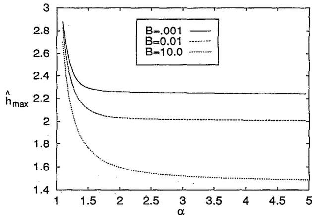
FIG. 3. Maximum coating thickness versus the shear-thinning exponent  $\alpha$  for several values of the stress ratio  $B$ . Here  $\tan \hat{\theta}_c = 1.0$ .
