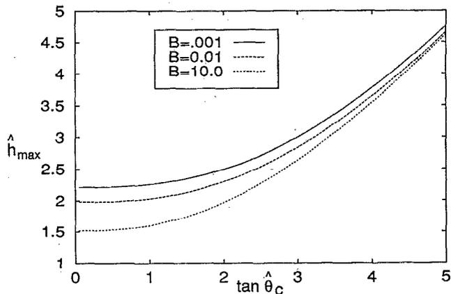
FIG. 4. Maximum coating thickness versus contact slope for several values of  $B$  and  $\alpha = 2$ .
