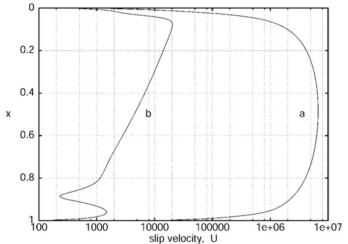
FIG. 5. Semi-log plot of early slip speed profiles for the nominal case. The initial concentration is  $G_0 = 500$ . Slip speeds at later times are much smaller. (a)  $t/T^* = 10^{-8}$ , (b)  $t/T^* = 8 \times 10^{-7}$ .
