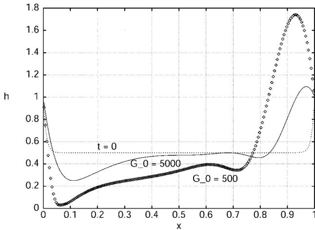
**FIG. 9.** Film profile comparison at  $t/T^* = 10^{-4}$  showing the effect of surfactant. Profiles are shown for  $G_0 = 500$  (symbols) and 5000. The initial ( $t = 0$ ) profile is also shown.
