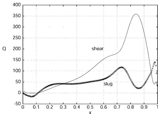
**FIG. 8.** Slug and shear flux components,  $G_0 = 500$ ,  $t/T^* = 10^{-4}$ . With surfactant, the shear flow component dominates at this instant in time.
