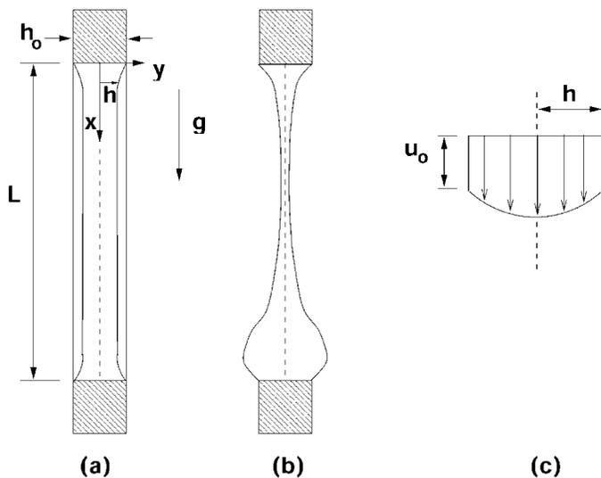
**FIG. 1.** Definition sketch for (a) the initial state of a soap film held vertically between upper and lower supports for two different initial profile shapes. (b) Sketch of the soap film at a later time showing gravity drainage. (c) The downward velocity profile is a linear combination of a slug flow at the interface slip velocity  $u_0$  and a parabolic shear flow.
