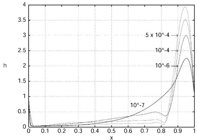
**FIG. 11.** Profiles at various times for a longer free film, corresponding to  $L = 2$  cm. All other physical parameters are the same as for the nominal case. Note that increasing  $L$  by a factor of 2 increases the time scale  $T^*$  by a factor of 16.
