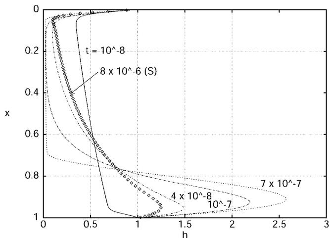
**FIG. 6.** Profiles without surfactant (lines). Comparison with surfactant (S) with  $G_0 = 500$  shown as symbols. The profiles, with and without surfactant, agree at  $t/T^* = 10^{-8}$ . Disjoining pressure prevents the no-surfactant profiles from going to zero thickness in finite time. The  $t/T^* = 7 \times 10^{-7}$  profile has reached steady state and is almost identical to the  $t = 4 \times 10^{-3}$  profile with surfactant shown above.
