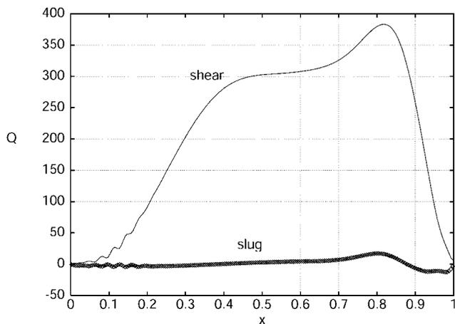
**FIG. 10.** Slug and shear flux components,  $G_0 = 5000$ ,  $t/T^* = 10^{-4}$ . The high level of surfactant immobilizes the surface.
