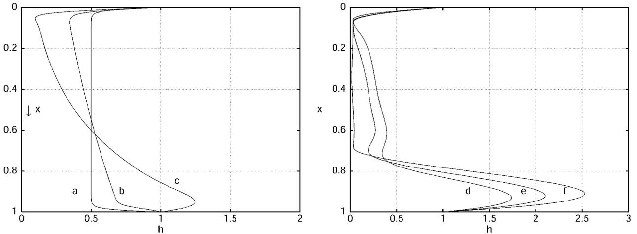
**FIG. 3.** Draining film profiles at various times for the nominal case with surfactant. See the text for parameter values. The initial profile is thinner in the middle region. (a)  $t = 0$ , (b)  $t/T^* = 10^{-8}$ , (c)  $t/T^* = 8 \times 10^{-7}$ , (d)  $t/T^* = 10^{-4}$ , (e)  $t/T^* = 5 \times 10^{-4}$ , (f)  $t/T^* = 4 \times 10^{-3}$ .
