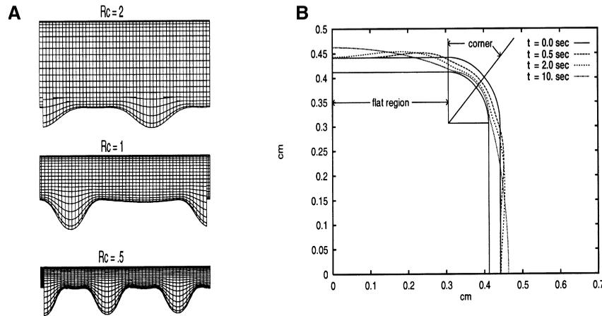
**Fig. 4** (A) Computed drop shapes hanging from horizontal cylindrical rods. The rod radius is given in units of the capillary length. (©Academic Press.) (B) The flow of Newtonian liquid away from an outside corner of radius 0.1 cm and the resulting profile at various times. The thickness of the coating layer is exaggerated for clarity. (With kind permission of Kluwer Academic Publishers.)
