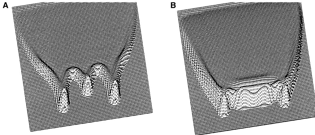
**Fig. 7** (A) Sagging of a Newtonian coating showing pronounced drip marks. (B) Sagging of a shear-thinning coating. Drip marks are less developed.
