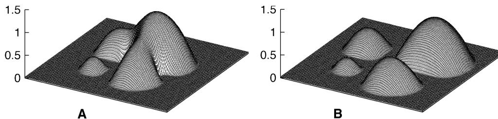
**Fig. 2** Time-dependent evolution of a drop placed near the center of a cross of poor-wetting material. (A)  $t = 0.35$  (dimensionless). (B)  $t = 0.70$ . (©Academic Press.)
