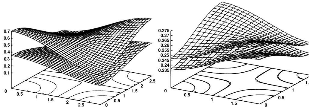
**Fig. 5** The leveling of an uneven coating with compositional changes; Coating height and “resin height” are shown. *Left:* At beginning; *Right:* Nearly dry coating. The Marangoni effect causes initial humps to dry as depressions. (Reprinted with permission from Ref. 44 ©1999 American Chemical Society.)
