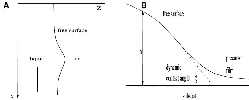
**Fig. 1** (A) Thin film flow down a windowpane. (B) Dynamic contact angle, apparent contact line and precursor film.
