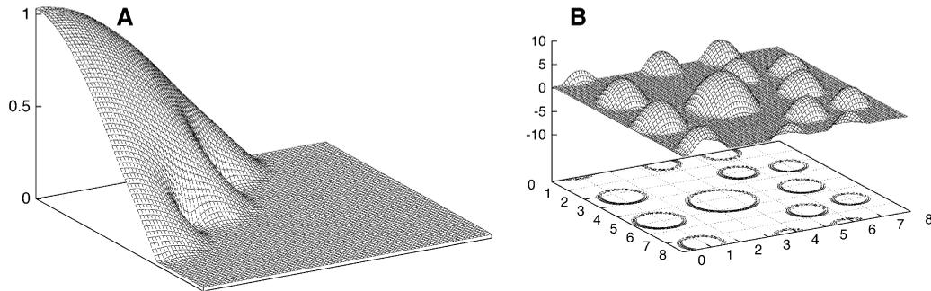
**Fig. 3** (A) The edges of a drop de-wet on “grease” patches. (Reprinted with permission from Ref. 28 ©1998 American Chemical Society.) (B) Modeling of spontaneous dewetting. An initially uniform liquid layer, perturbed, breaks into long ridges and then into isolated droplets.
