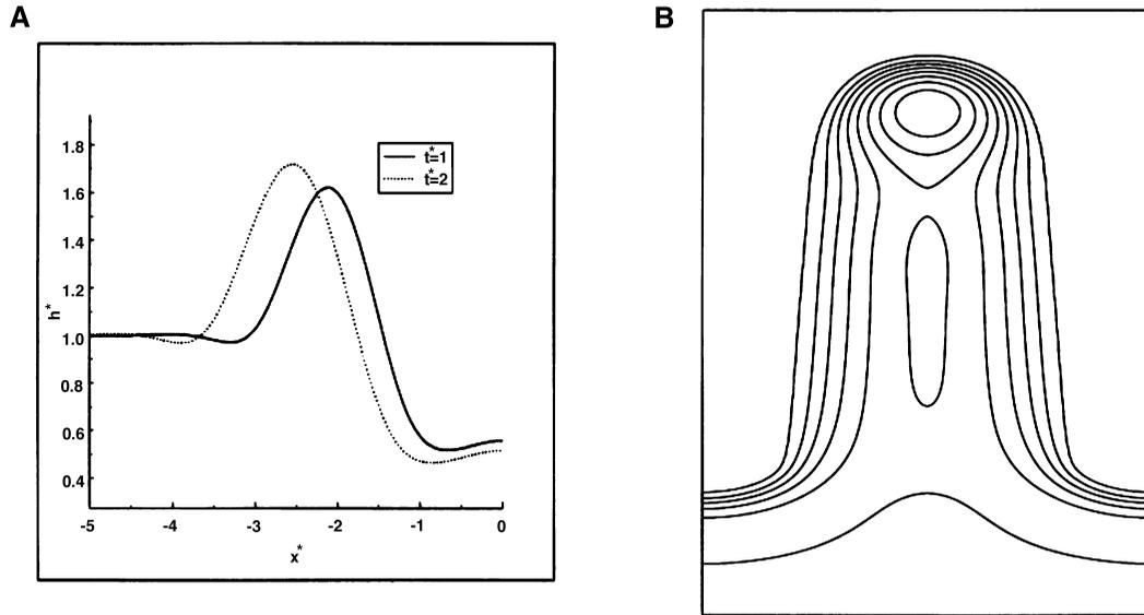
**Fig. 6** (A) Marangoni drying flow induced by surfactant. (B) Simulation of thin-film “fingering” driven by a temperature gradient.
