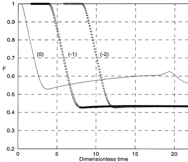
Figure 5. Cell fill fraction  $F$  vs. time for three identified cells, hexagonal pattern. The (0) cell lies at the origin  $(x, y) = (0, 0)$  at time  $t = 0$ . Cells (-1) and (-2) lie in the following two rows, respectively.
