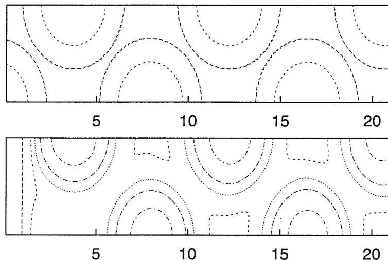
Figure 7. Contour plots of the gravure (top) and coating surface (bottom). Diamond pattern; time = 25. Contour levels for the gravure are  $-0.5$  and  $-0.001$ ; for the coating surface, they are  $-0.5$ ,  $-0.2$ ,  $0$ ,  $0.2$ ,  $1$ .
