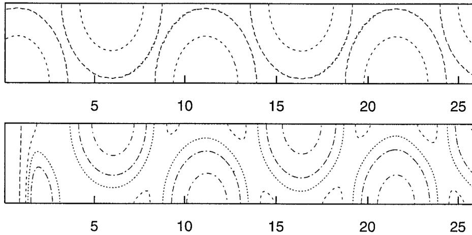
Figure 8. Contour plots of the gravure (top) and coating surface (bottom). Hexagonal pattern; time = 32. Contour levels for the gravure are  $-0.5$  and  $-0.001$ ; for the surface, they are  $-0.5, -0.2, 0, 0.2, 1$ .
