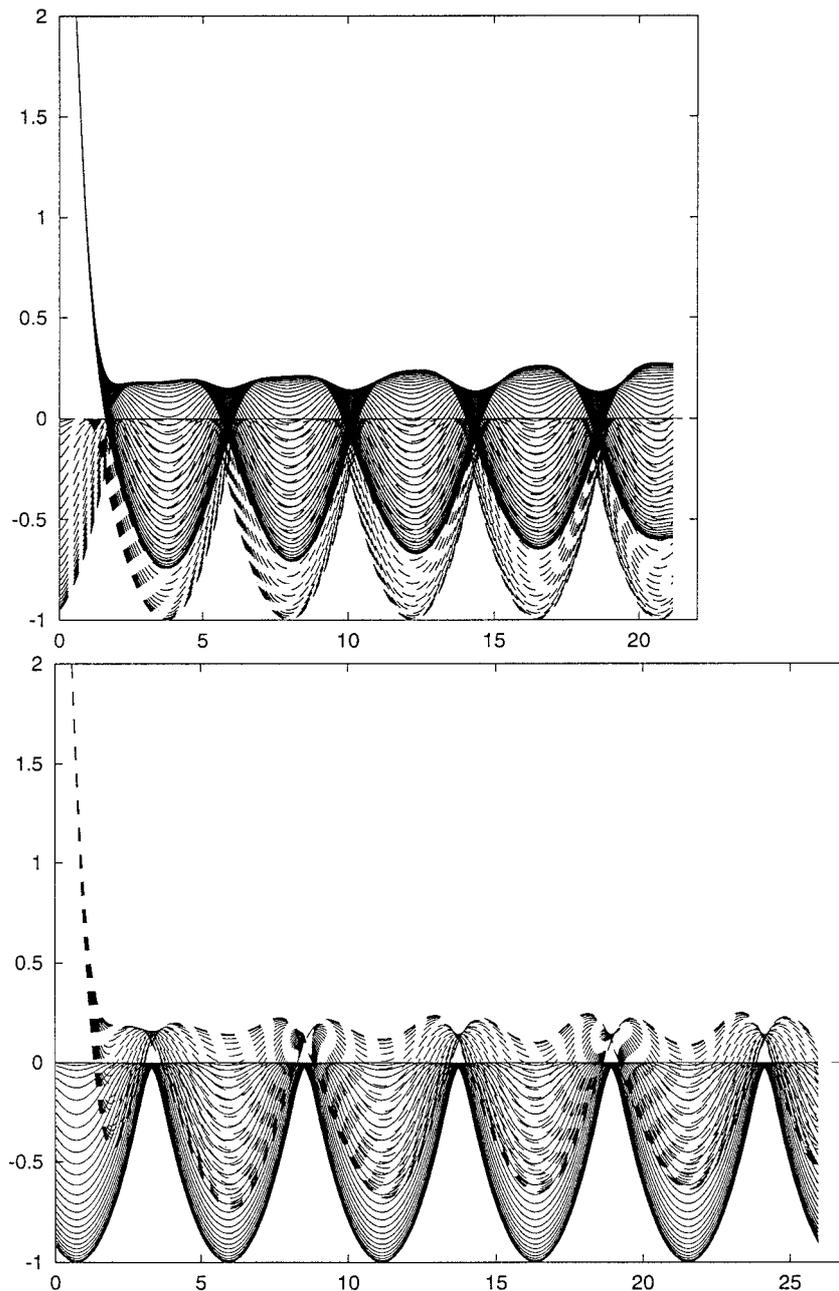
*Figure 9.* Edge views of the gravure and the coating. Top: diamond pattern, time = 25. Bottom: Hexagonal pattern, time = 32. Note the rise in meniscus height within the cells as one moves to the right. This indicates refilling.
