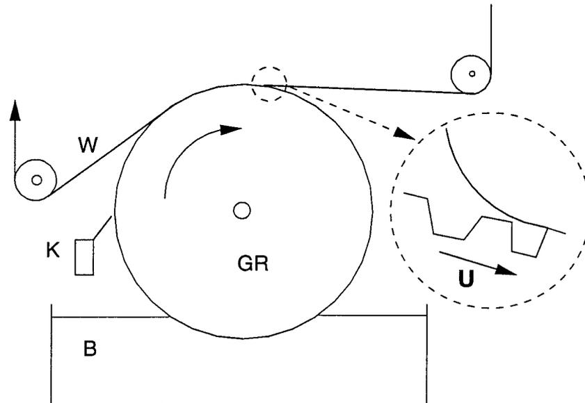
Figure 1. Schematic diagram of a roll coater that removes liquid from a bath  $B$  and transfers it to the moving web  $W$ . The small gravure cells are seen in enlargement in the inset where the liquid-air meniscus is also shown. This paper deals with flow in the liquid region bounded by the gravure and the meniscus.
