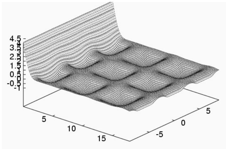
Figure 11: A frame in a time-dependent calculation of the withdrawal of liquid from gravure cells. The liquid meniscus is “pinned” at the left boundary and the gravured substrate (not shown) is moving to the right.<sup>23</sup>
