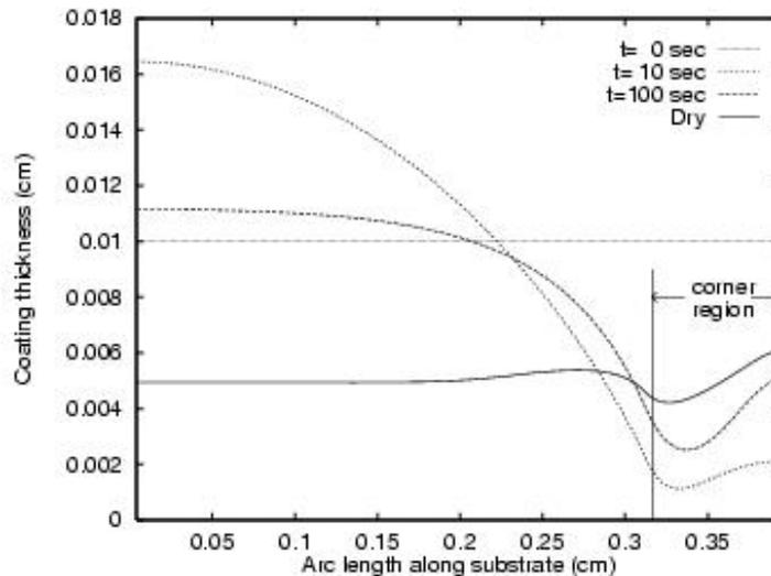
Figure 10: Coating thickness versus position and time for the substrate shown in Fig. 9 ("Un-wrapped"). Here drying is considered and the drying rate is optimized so as to use Marangoni forces to "pull back" the coating after the initial displacement by capillary forces.<sup>20</sup>
