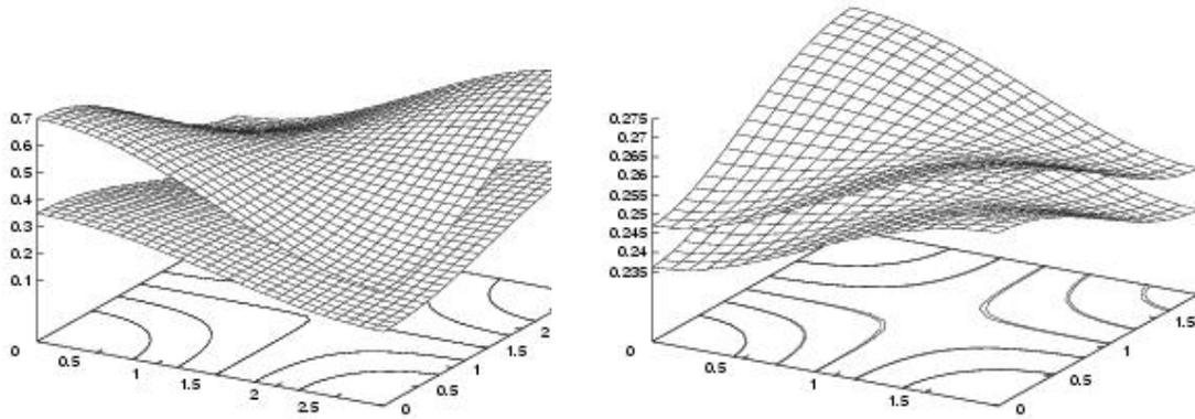
Figure 12: Leveling of an uneven coating with compositional changes; The coating height and “resin height” are shown. Left: Initial state; Right: The coating is almost dry. Maragoni effect causes initial humps to dry as depressions.
