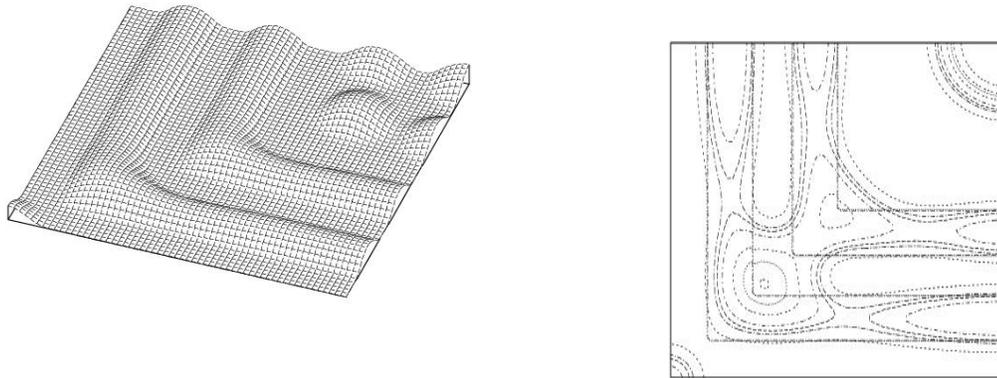
Figure 7: Modeling result for vapor deposition on a mixed-wettable substrate, as used to produce a microelectric circuit. Left: The liquid forms continuous conducting channels and isolated droplets, as seen in the experiments of Gau *et al*<sup>17</sup>. Right: Contour plot of modeling result at a later time, after more liquid has been deposited. The liquid overflows near the corner, bridging the gap between the two L-shaped regions and causing a short circuit.
