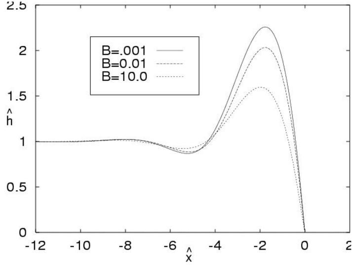
Figure 15: Coating flow of an Ellis fluid liquid on a vertical wall.<sup>31</sup> The total force at the contact line is finite because of shear-thinning effect. Curves show coating profiles for several values of the stress ratio  $B$  in Eqn. (6.3).
