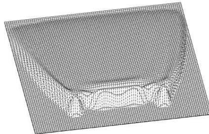
Figure 17: Sagging pattern for a shear-thinning coating. Drip marks are much less developed.
