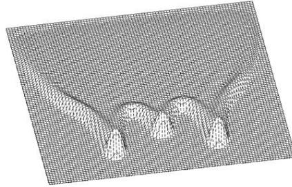
Figure 16: Sagging pattern for a Newtonian coating showing pronounced drip marks.
