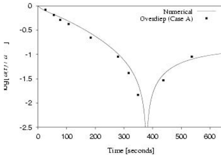
Figure 13: Comparison of experiments<sup>25</sup> and model prediction<sup>24</sup> for the amplitude of a initial bump in a drying layer of alkyd paint. Surface tension gradient effects, that develop as the mixture dries, cause the amplitude to first fall and then rise.
