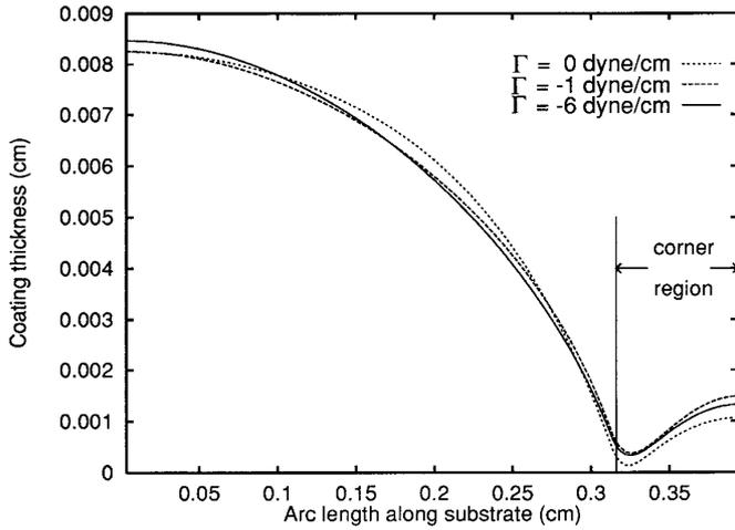
**FIG. 9.** Final dry coating profiles for various values of  $\Gamma$ . Here  $\Delta\sigma = 0$ ,  $D^{(s)} = 1.0 \times 10^{-5} \text{ cm}^2/\text{s}$ ,  $D_b = 0.0 \text{ s}^{-1}$ ,  $\alpha = 0.5$ , and  $E_0 = 1.36 \times 10^{-5} \text{ cm/s}$ , corresponding to a dry time of 14.0 min. Dimensionless parameters are  $\hat{E}_0 = 1.45$ ,  $\hat{D}^{(s)} = 0.108$ ,  $\hat{D}_b = 0.0$ , and  $3.63 \times 10^{-3} \leq -\Gamma/\sigma_0 \leq 2.18 \times 10^{-2}$ .
