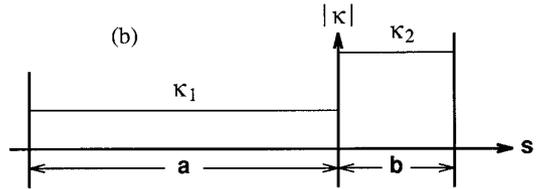
**FIG. 2.** (a) A substrate composed of two circular arcs with a continuous tangent. (b) The corresponding curvature distribution.
