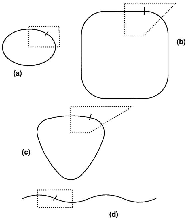
**FIG. 3.** Similar bodies for coating flow behavior,  $a = b$ ,  $a(\kappa_2 - \kappa_1) = \pi/4$ . The location of the curvature discontinuity and the unit cell are shown for each body. The coating may be either outside or inside. Parameter values are (a)  $a\kappa_1 = \pi/8$ ,  $a\kappa_2 = 3\pi/8$ ; (b)  $a\kappa_1 = 0$ ,  $a\kappa_2 = \pi/4$ ; (c)  $a\kappa_1 = \pi/24$ ,  $a\kappa_2 = 7\pi/24$ ; (d)  $a\kappa_2 = -a\kappa_1 = \pi/8$ .
