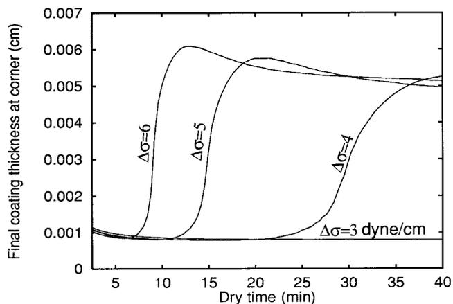
**FIG. 8.** Comparison of final dry corner thickness ( $h$  at  $s = 3.93$  cm) for various values of  $\Delta\sigma$ . Here  $\alpha = 0.5$ , corresponding to a dry time of  $t_{\text{dry}} = 1.14 h_0/E_0$ ,  $\Gamma = 0.0$  dyn/cm,  $A = 15.0$ , and  $K_D^{(j)} = 2 \times 10^{-5}$  cm<sup>2</sup>/s. Dimensionless parameters are  $0.5 \leq \hat{E}_0 \leq 8.08$ ,  $\hat{K}_D^{(j)} = 0.2153$ , and  $0.109 \leq \Delta\sigma/\sigma_0 \leq 0.218$ .
