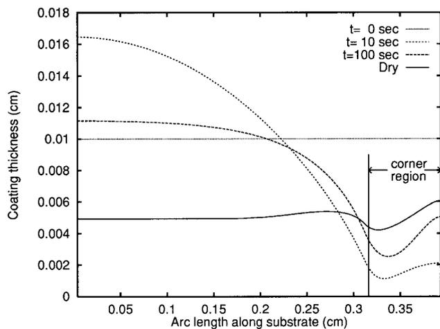
**FIG. 6.** Sequence of coating profiles for model coating with  $\alpha = 0.5$ , and  $E_0 = 1.36 \times 10^{-5}$  cm/s, corresponding to a dry time of 14.0 min. Here  $\Gamma = 0.0$  dyn/cm,  $\Delta\sigma = 6.0$  dyn/cm,  $A = 15.0$ , and  $K_D^{(r)} = 2 \times 10^{-5}$  cm<sup>2</sup>/s. Dimensionless parameters for this case are  $\hat{E}_0 = 1.44$ ,  $\hat{K}_D^{(r)} = 0.215$ , and  $\Delta\sigma/\sigma_0 = 0.218$ .
