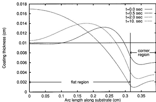
**FIG. 5.** Coating height variation versus arc length for the same case as described in the legend to Fig. 4.
