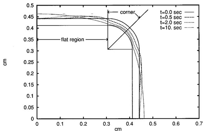
**FIG. 4.** Reference case for flow away from an outside corner for a nonevaporating Newtonian liquid of constant surface tension. Here the corner radius is 0.1 cm. The coating profiles are shown at various times. Note that the thickness of the coating layer has been magnified by a factor of 3 for clarity. Dimensionless parameters for this case are  $a/b = 4$ ,  $M = 100$ , and  $h_0/a = 0.0318$ .
